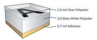
to permanently bond to high and low surface energy plastics, stainless steel, glass, and nylon. The label has good resistance to general purpose and household cleaners, mild acids, oil and water. Expected exterior life is up to two years.
